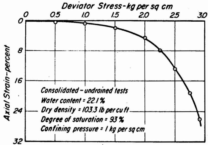
Typical stress vs strain relationship for compacted silty clay.
