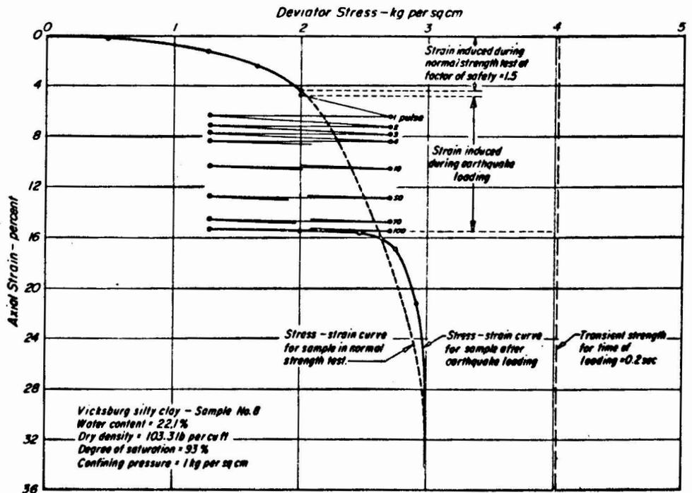
Fig. 19 - STRESS vs STRAIN RELATIONSHIP IN SIMULATED EARTHQUAKE LOADING TEST ON SILTY CLAY.
