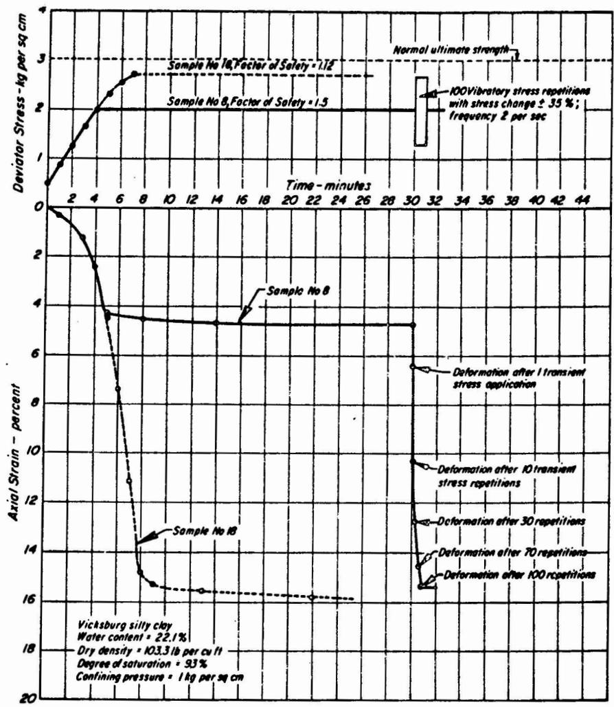
Fig. 18 - CHANGES IN STRESS AND DEFORMATION WITH TIME DURING SIMULATED EARTHQUAKE LOADING TEST ON SILTY CLAY.
