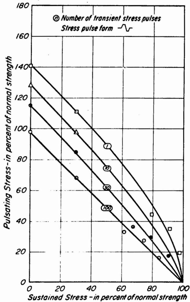
Fig.20-COMBINATIONS OF SUSTAINED AND PULSATING STRESS INTENSITIES CAUSING FAILURE - COMPACTED VICKSBURG SILTY CLAY.
