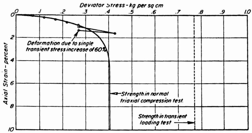
Fig. 17a - SOIL DEFORMATION DUE TO A SINGLE TRANSIENT STRESS PULSE
