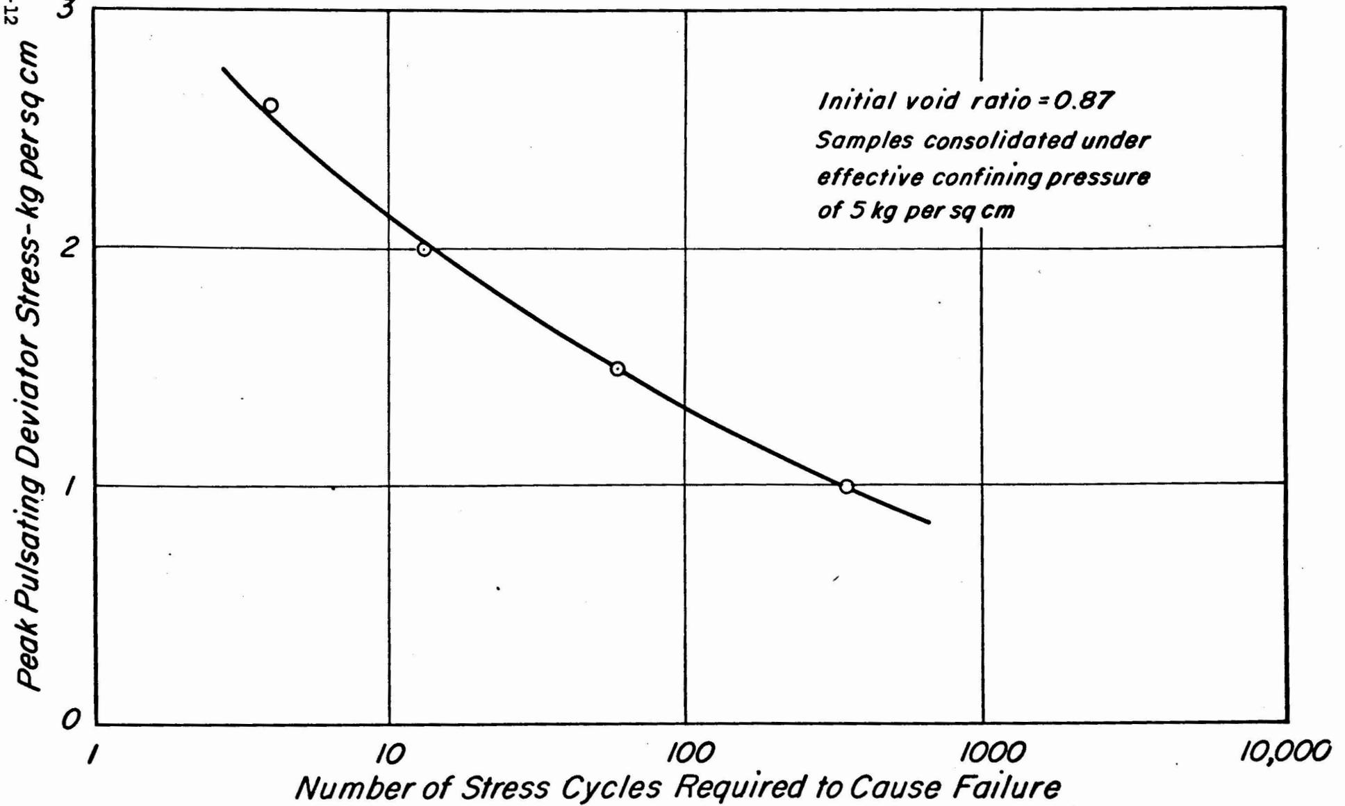
Fig.15- RELATIONSHIP BETWEEN CYCLIC STRESS AND NUMBER OF STRESS CYCLES CAUSING FAILURE.
